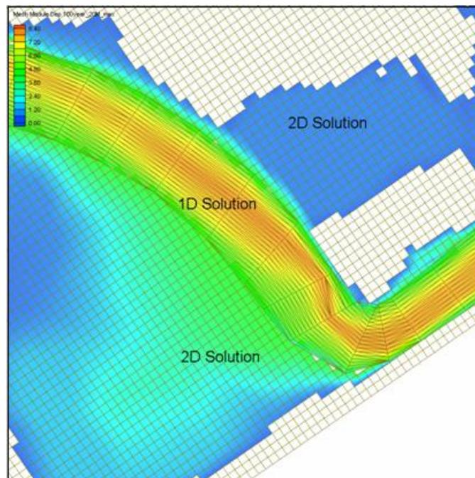
Figure 16 2D and 1D TUFLOW Solution
