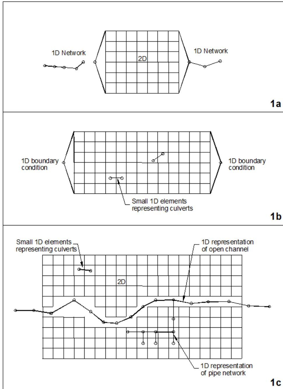
Figure 2 1D/2D linking mechanisms<sup>2</sup>
