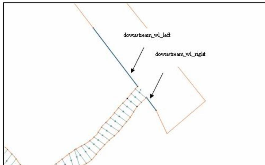
Figure 13 Location of downstream boundary condition arcs
