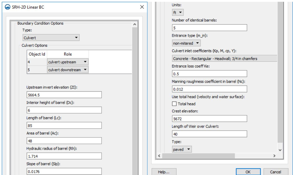
Figure 4 Culvert Parameters
