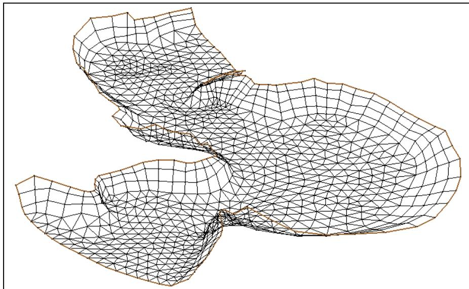
Figure 12 Mesh with interpolated elevation
