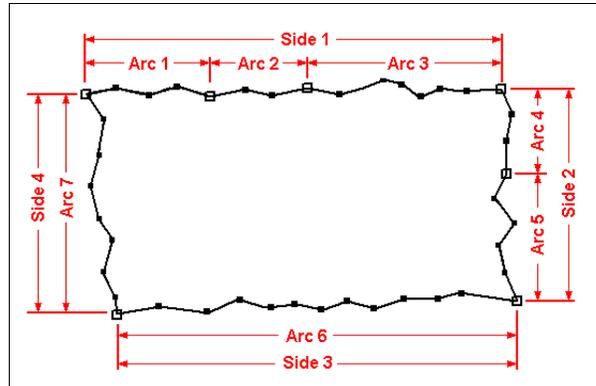
Figure 7 Four sides required for a rectangular patch
