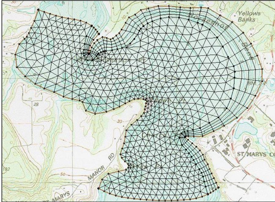
Figure 9 Mesh with both paved and patch methods
